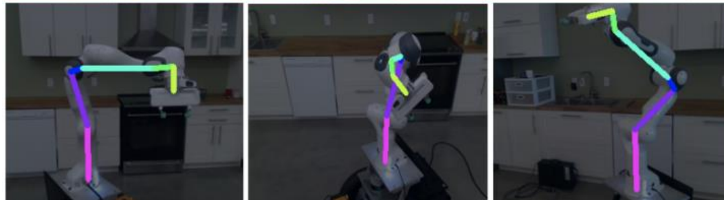
Projected skeleton based on estimated robot pose:
